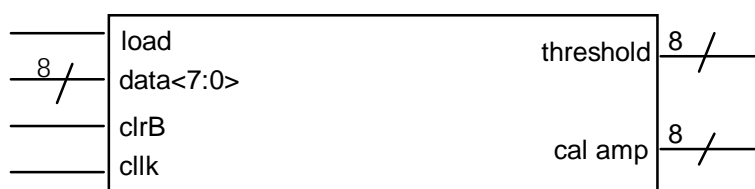
Figure 3.12. Threshold/Calibration DAC Register Inputs/Outputs.
